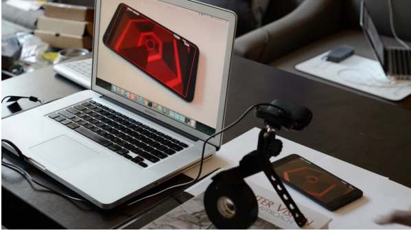
Figure 4. Experimental setup. The phone, right, is filmed by the webcam, which is connected to the laptop. In this test, the laptop is drawing the extracted bounding box on the raw webcam footage.
